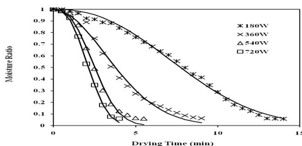
Figure 3. Variation of moisture ratio with drying time of *Pandanus* leaves at different power levels
